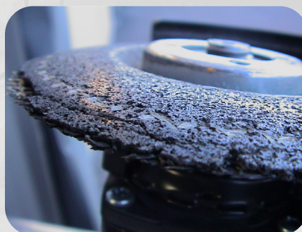
Figure 3. Mass imbalance of grinding disk
